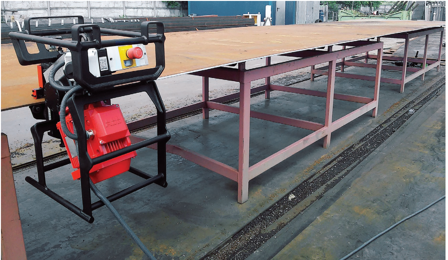
ABM-14 runs along a plate automatically
