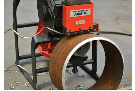
Oval workpiece and pipe beveling
