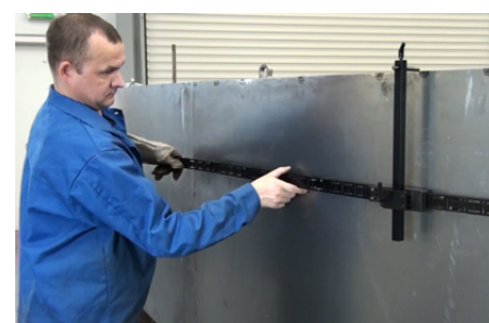
Guide adjustment tool to position the track parallel to the edge Product code: UST-0466-53-00-00-0
